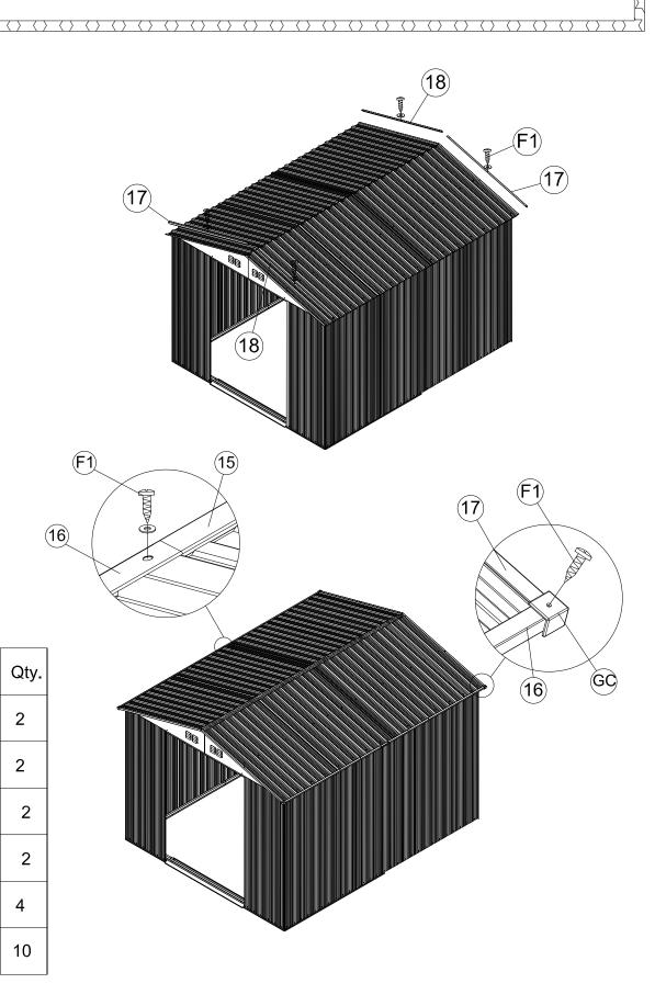
Place two pieces of the roof flashing center (19) on top of the roof panels, Line up the holes and secure them with (F1) screws with washers. Then slide the flashing end cap (GE) to the front & back top of the roof and secure with (F1) screws with washers. See figures below.
