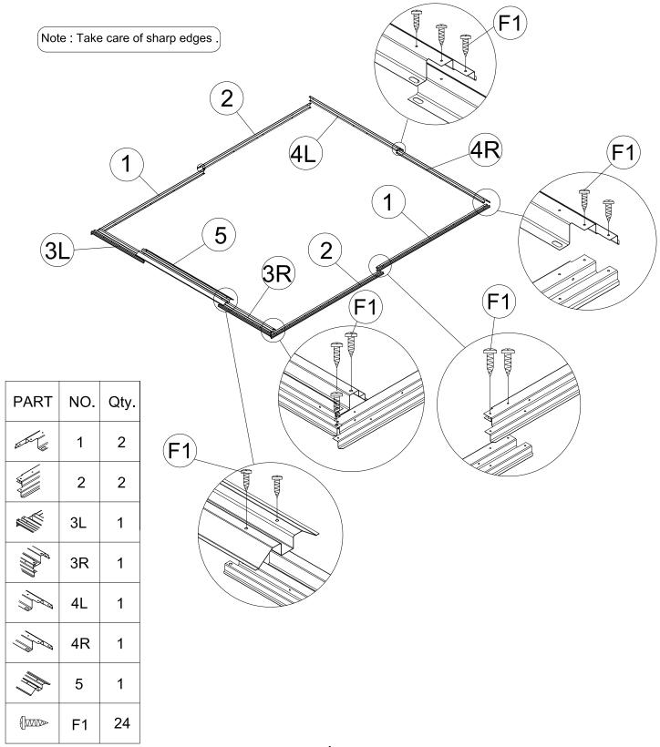
Place the wall panel (P1),(P2),(P3),(P4),on the base bar (1), (3L),(3R), (4L),and (4R) as showing .Side wall of the shed line up the Holes With base bar.
