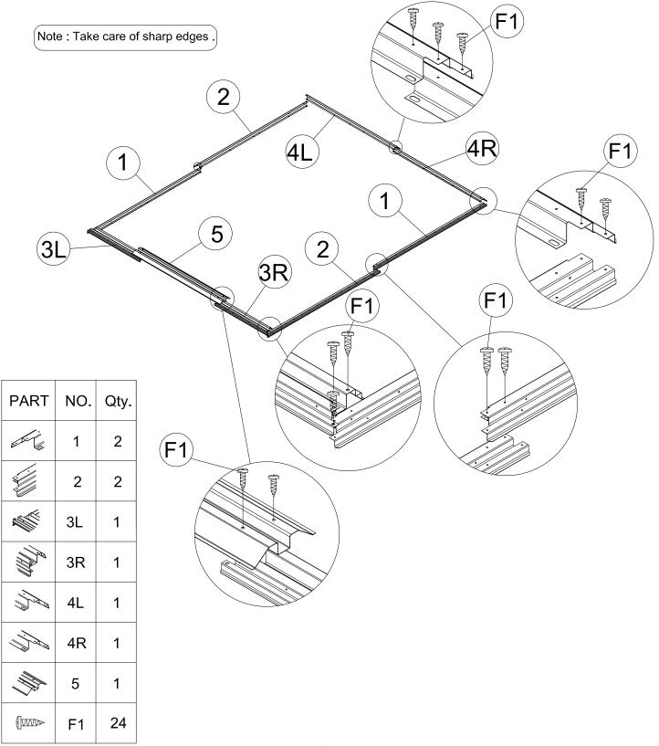
Place the wall panel (P1) and (P2) on the base bar (3L) (3R),(4L)and (4R) as showing .Side wall of the shed line up the Holes With base bar.Secure with (F1). Screws with washers from outside.
